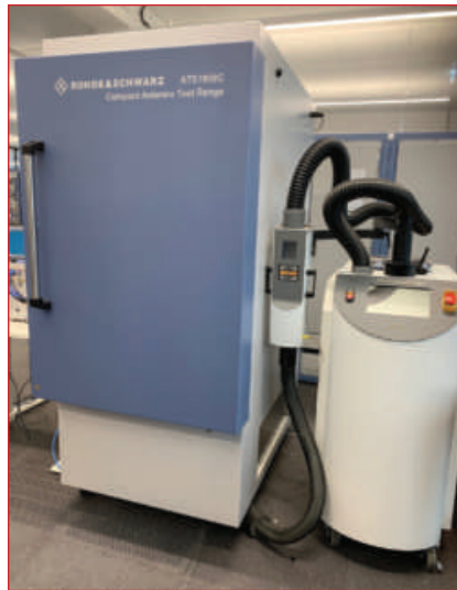
▲ Fig. 3 ETC OTA test system (R&S®ATS1800C) with a commercial Thermo-stream.
